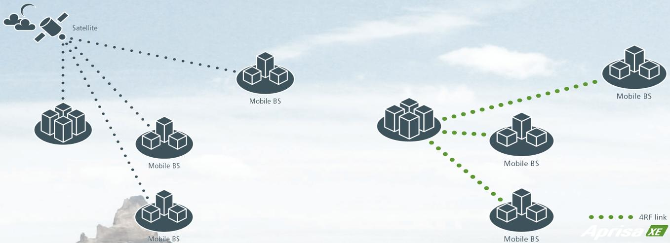
Satellite latency can impact network performance, particularly for time-sensitive voice calls. Deployment can be time-consuming and difficult, requiring large antennas, and with the need for a clear view of the sky, obtaining the relevant roof rights can be problematic. Weather conditions can also cause signals to fade significantly.
